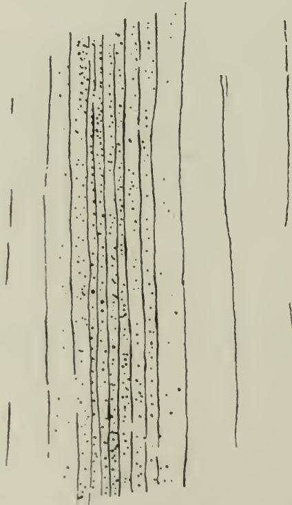
FIG. 4. Lode fissure formed by the replacement of plates of rock in between multitudes of parallel fractures. Fissures decrease in number from centre of disturbance outward.
